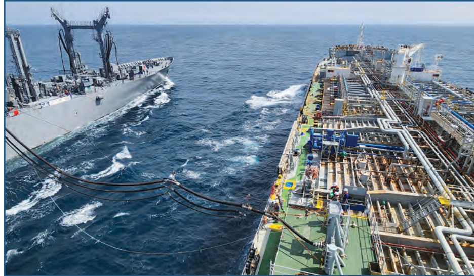
Japan Maritime Self-Defense Force oiler JS Hamana connects its fuel lines to the Badlands Trader , operated under Military Sealift Command charter by USMMI.
